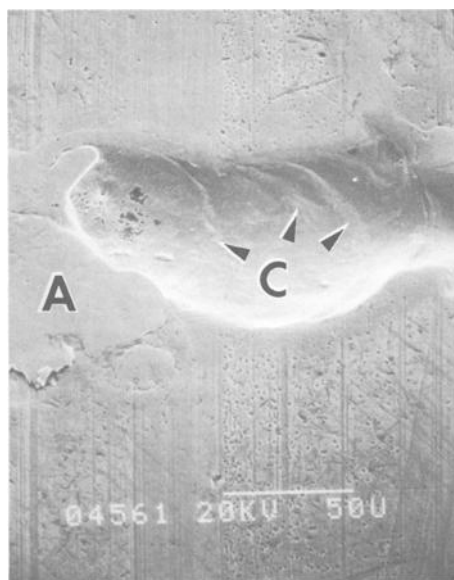
FIG. 5—The brightly reflecting base of a roller surface pit showing flow marks.
