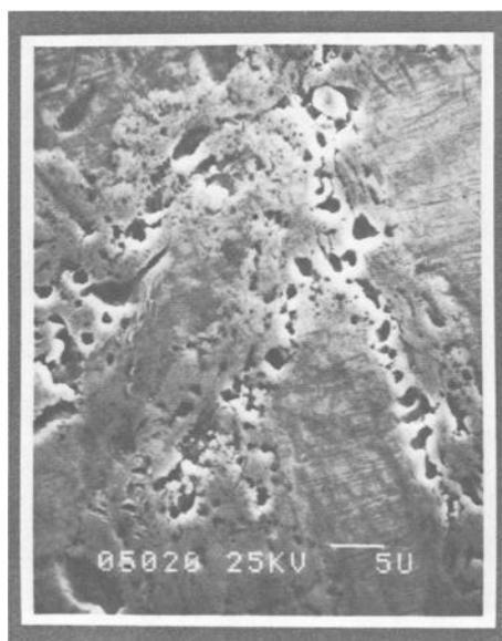
FIG. 6—Micropit stringers fantailing away from a large pit which is out of view at top.
