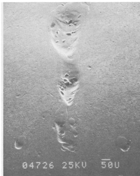
FIG. 3—Surface pits in a roller showing both longitudinal and lateral placement of pits.
